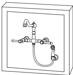
10. Once installation is complete, turn the main water supply back on from underneath your sink. Check for any leaks underneath.
