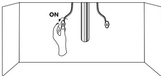
11. Remove the aerator from the spout and turn the faucet on. Ensure that both hot and cold water are running properly, and check for any leaks. Allow the water to flow for approximately 60 seconds to remove any dust or sediment within the water lines. Reattach the aerator and turn on the sprayer. Allow the sprayer to run for another 60 seconds, and check for any leaks.
