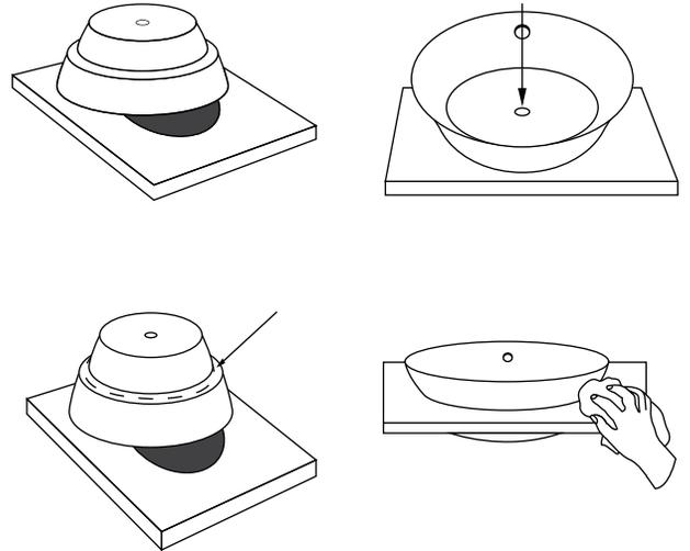
6. Let the assembled vanity sit for 24 hours to allow all the silicone sealant to fully dry. Once dry, proceed to the installation of your faucet and drain assemblies.
