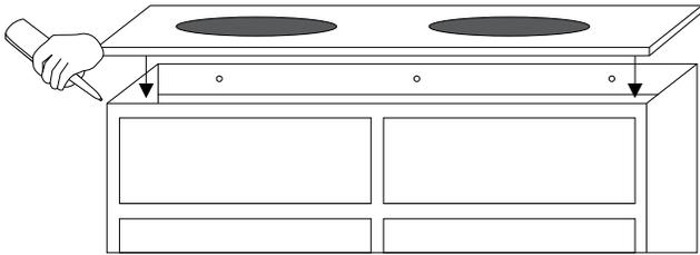
2. With assistance from another person, slowly and carefully set the counter top onto the vanity cabinet. Once positioned, press firmly into place. Wipe away any excess sealant using a damp cloth.
