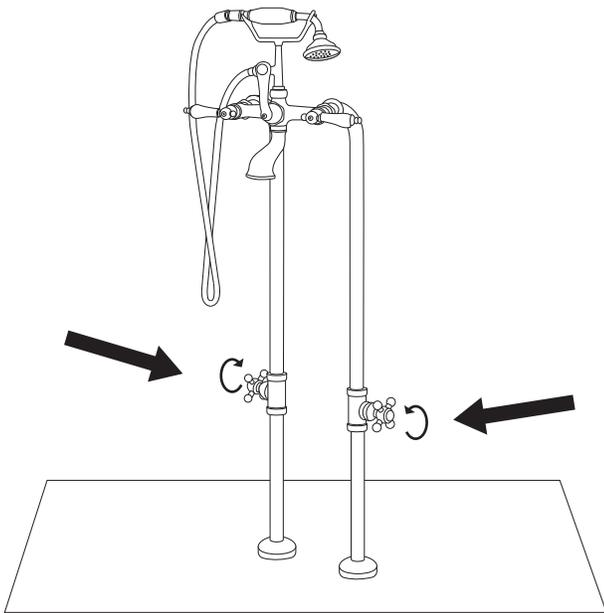
12. Turn the faucet on and allow the water to run through the spout for approximately 60 seconds. Divert the water to the hand shower and allow the water to flow for another 60 seconds. Check to make sure that all connections are tight, and there are no leaks.
