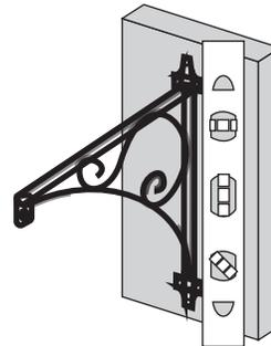
3. While holding the bracket in place, mark the location of the mounting holes with a pencil or marker.
