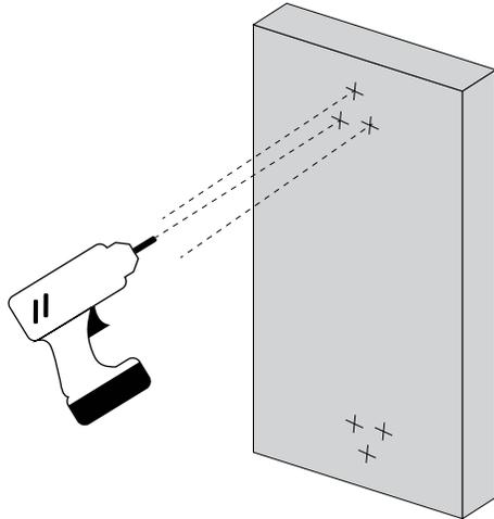
5. Attach the bracket to the wall using the provided mounting screws. Be careful not to overtighten, which could strip or break the screw.
