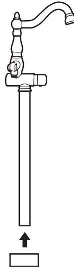
4. Attach the mounting bracket by threading it onto the base of the faucet. Hand tighten firmly. Position the faucet at its desired location, then mark the location of the mounting holes on the floor. Set the faucet aside.
