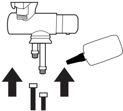
2. Feed the water lines through the faucet body and attach the spout by threading it onto the body.
