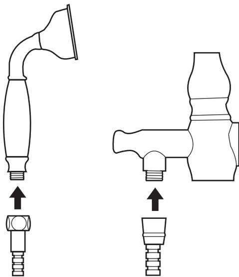
11. Once installation is complete, turn on the main water supply. Remove the aerator from the spout and turn the faucet on. Allow the water to flow for 60 seconds to remove any dust or loose sediment within the water lines. Check for any leaks, and that hot and cold water are running appropriately. Divert the water to the hand shower and allow the water to flow through the hose for approximately 60 seconds.
