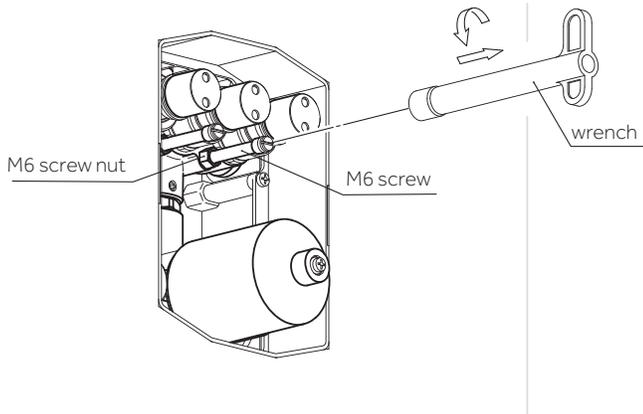
13. Place the positioning bar against the wall as shown. Adjust the height of the M6 screw until it meets the surface of the bottom of the positioning bar. Then, tighten the M6 screw nut with the wrench.
