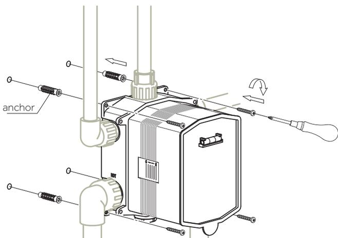
7. Connect the hot and cold water feed lines to the installed valve.
