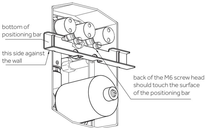
14. Turn on the switch. Place the positioning bar against the wall. Adjust the height of the cap so that the front side of the cap is even with the front side of the positioning bar.
