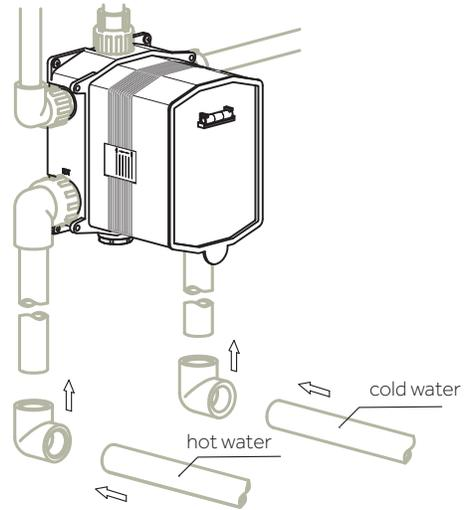
8. Remove the protective cover and turn off the switch. Flush the water lines and check for leaks.
