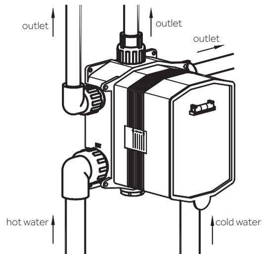
4. Hold the valve up to its desired installation location. Use the level on the mounting box to ensure it is straight, then mark the location of the valve's mounting holes as shown below.
