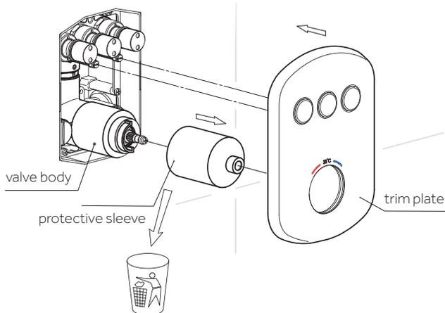
18. Press the buttons on the valve to ensure they work properly with the fitment of the trim plate. When a button is turned on, it should protrude approximately 1/4" from the trim plate.
