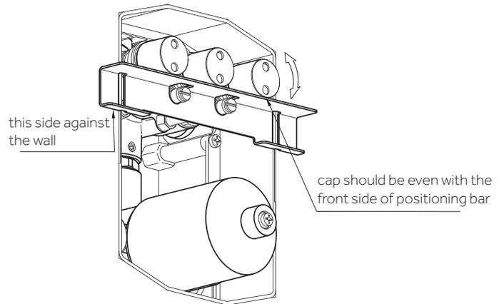
15. Replace the M6 screws with the shorter M6 screws. Then, adjust the screws as indicated in step 12.
