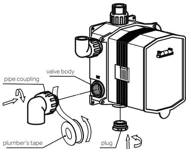
3. Connect all inlet and outlet pipes as shown in the diagram below.
