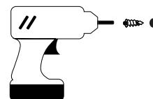
4. Mount hanger bolts to the wall, leaving approximately 1-1/4" (3.2cm) of each bolt exposed.
