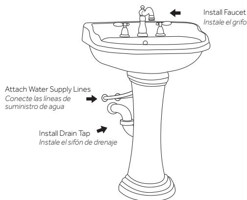
8. Complete the installation by applying a thin bead of silicone around the back of the sink, where it meets the wall. This will prevent water from getting behind the sink, which could damage drywall. If desired, apply another thin bead of silicone around the base of the pedestal, where it meets the floor.
