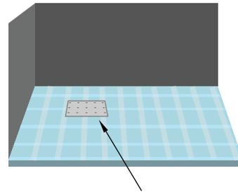
**Note:** Be sure to leave room for final thinset and tile application. The top of the drain should be level and 1/16" below the adjacent tile.
