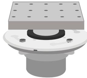
3. Place pea gravel over the drain flange coupling weep holes and around the perimeter to prevent mortar from filling and blocking the holes.
