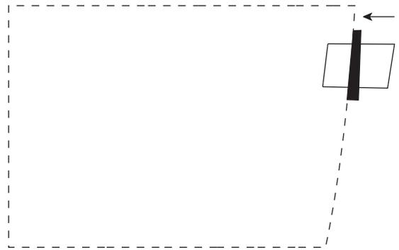
8. Once the overflow assembly and gaskets are properly aligned, the overflow assembly will need to be cut to size. Hold the overflow assembly in place. Measure 1/2" from the outside gasket and mark this location on the overflow assembly's threading.
