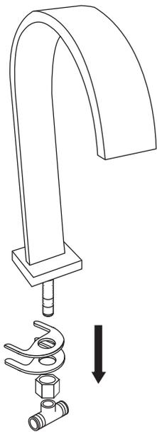
3. Set the spout into the center mounting hole. From beneath the countertop, slide the rubber gasket followed by the metal washer back onto the threaded mounting post. Hand tighten the lock nut, then finish tightening using an adjustable wrench.
