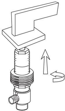
6. Set the removed handle into the right-side faucet hole. From beneath the counter top, insert the valve stem into the right-side faucet hole. Hand-tighten the stem into the handle base firmly. Hand tighten the blue lock nut until the stem is secure, then finish tightening using a basin wrench.
