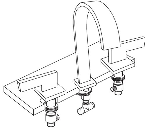
8. Use the provided braided water lines to connect each stem to the spout's T-connector, as shown. Apply thread sealant or plumber's tape to each threaded connection. Use an adjustable wrench to tighten, but be careful not to overtighten.
