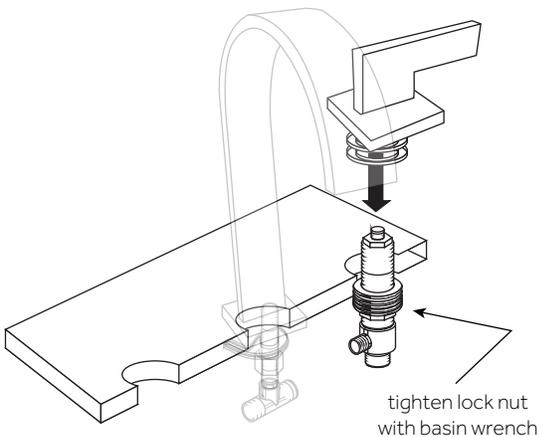
7. Repeat steps 5 & 6 to install the 'hot' valve stem into the left-side faucet hole.
