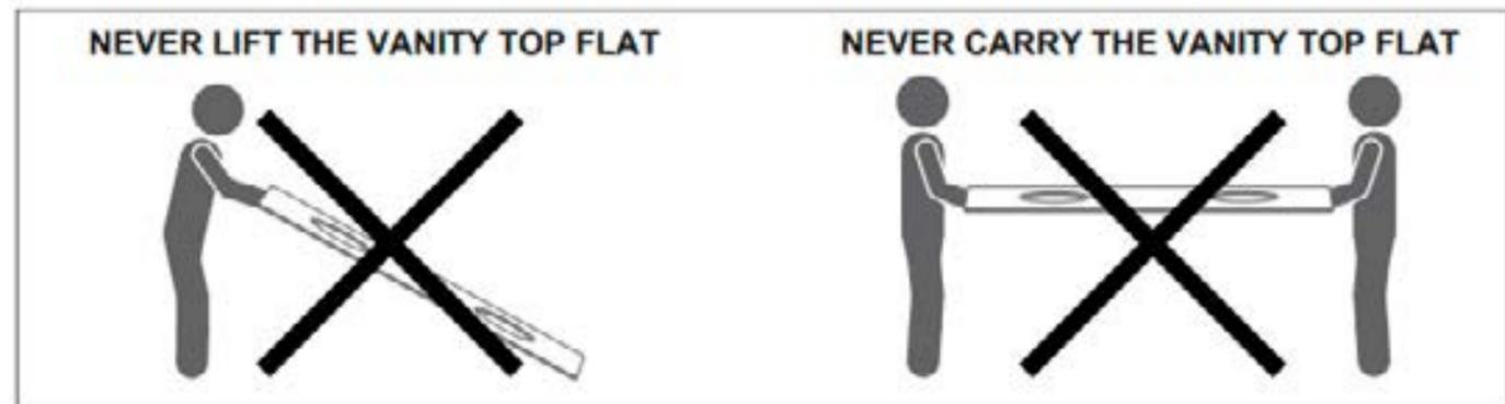
1. Lift the vanity top from the front edge, bringing to a vertical position, while keeping the back edge in the box.
