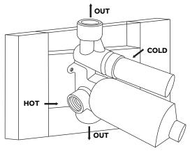
3. Route, assemble, and connect all in-wall piping to and from the shower valve. Make connections appropriately depending upon the type of pipe that is being used. For copper pipe, soldering will be required and should be completed by a licensed plumber. Apply plumber's tape to any threaded connections if applicable. Install any wood blocking that is necessary to support the piping and valve.
